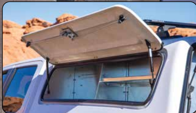
3 point locking side doors, shown with galvanized steel tool boxes
