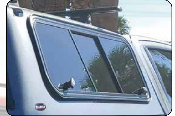
Optional side Windoor with Slider provides ventilation without opening the entire window
